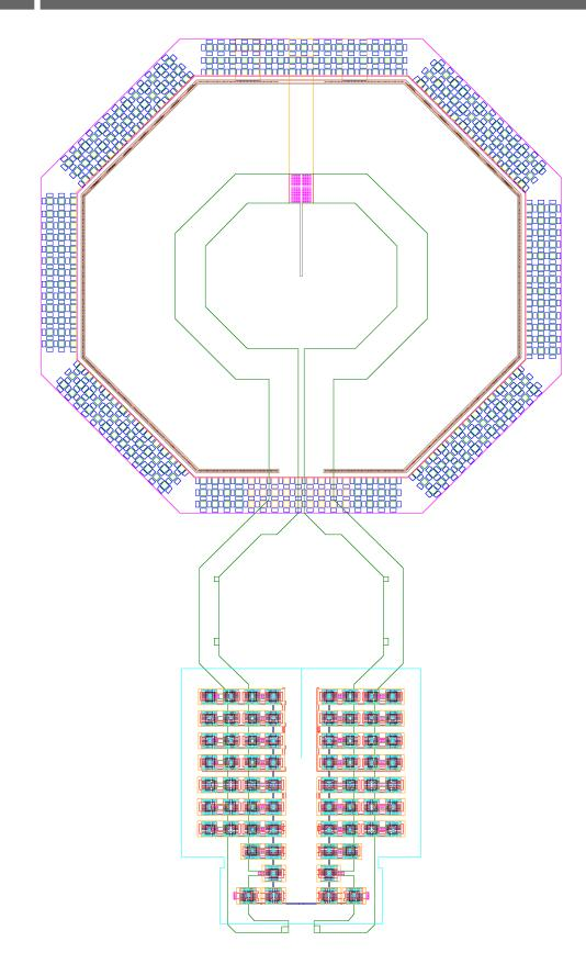
VCO full-wave extraction, with inductor, capacitor bank and interconnect on a TSMC 90nm process
