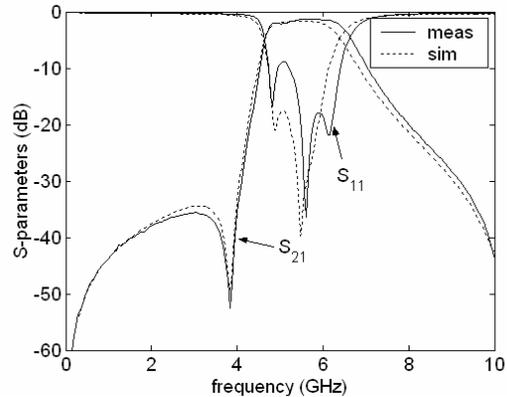
Figure 5: Measured and simulated characteristics for the 802.11a bandpass filter shown in Fig. 3.
