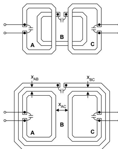
**Figure 2: Physical implementations. The upper diagram shows the arrangement with three identical inductor rings, the lower with a larger middle stage.**
