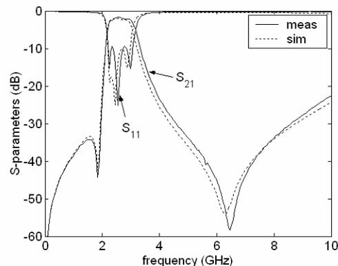
Figure 5: Measured and simulated characteristics for the 802.11b bandpass filter shown in Fig. 3.
