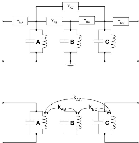
**Figure 1: Top: general circuit configuration for a three-stage top-coupled bandpass filter. Bottom: an alternative configuration in which the coupling is by mutual inductance.**
