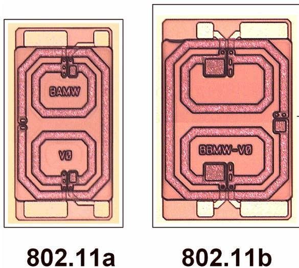
Figure 3: Micrographs of two example bandpass filters.
