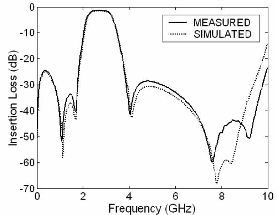
Fig. 9. Measured and simulated characteristics of the flip-chip 802.11b band-pass filter.
