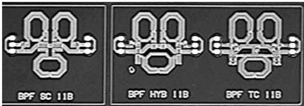
Fig. 5 Micrograph of three bandpass filters using different coupled-resonator topology, implemented in thin-film IPD technology on silicon substrates.
