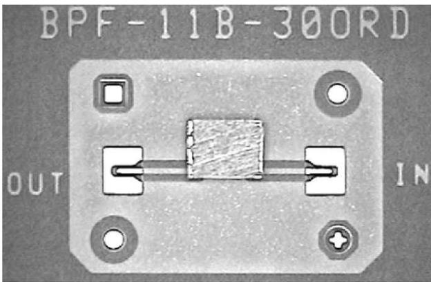
Fig. 8. Test board configuration, showing the IPD mounted face-down using flip-chip attachment.
