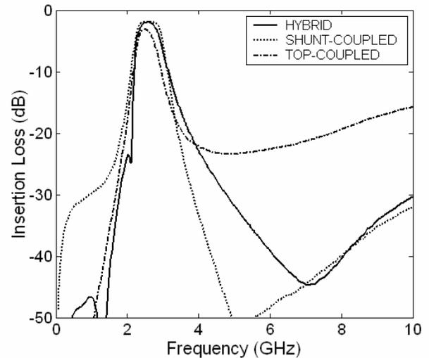
Fig. 6. Measured characteristics of the wafer-probe filters.
