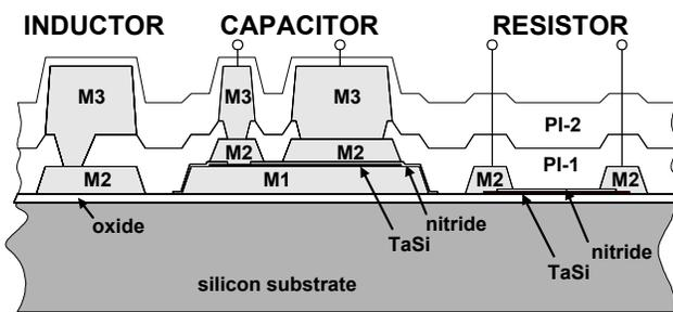
Fig. 1. Thin-film integrated passive device (IPD) structure.
