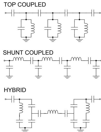
Fig. 4. Several alternative 3<sup>rd</sup>-order band-pass filter topologies.
