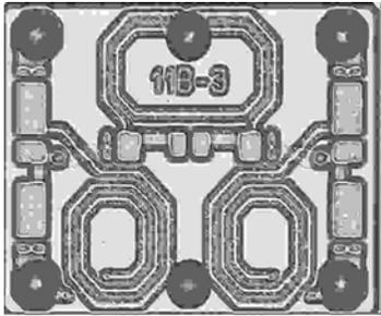
Fig. 7. Micrograph of a 3<sup>rd</sup>-order flip-chip 802.11b band pass filter using the hybrid circuit topology.
