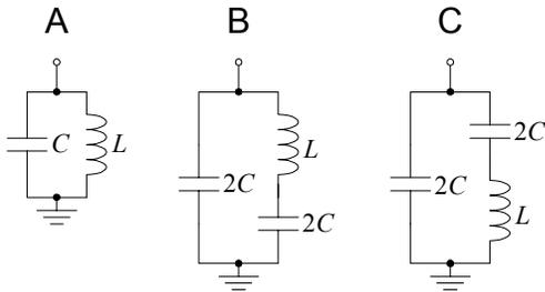
Fig. 3. Resonator circuits.
