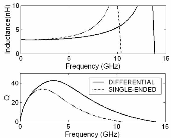
Fig. 2. Comparison of simulated inductance and Q for a typical example IPD inductor in differential and single-ended operation.
