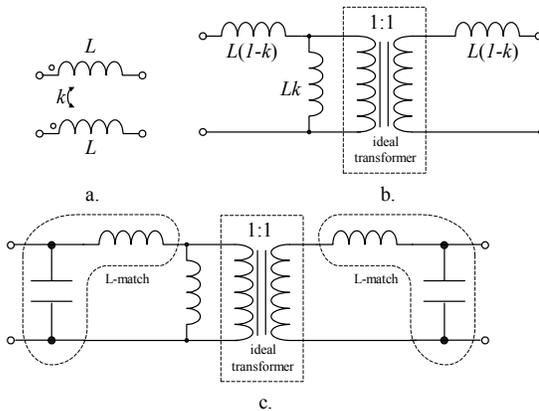
**Figure 2: a) basic coupled inductor , b) equivalent circuit, and c) coupled inductor with shunt resonating capacitors, showing L-match elements.**
