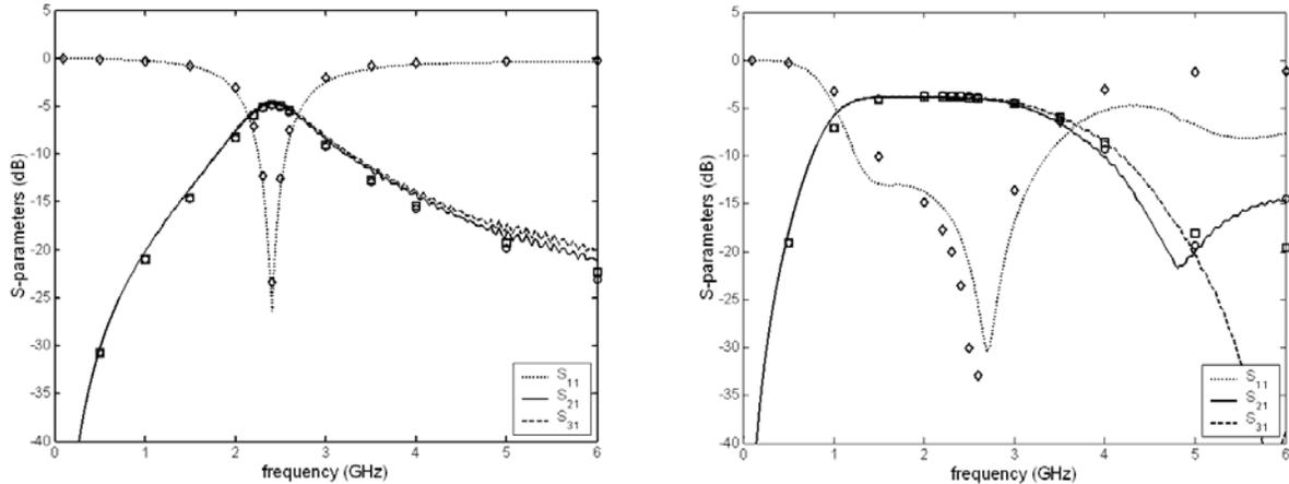
**Figure 6 Measured and simulated S-parameters for balun-1 (left) and balun-5 (right). Port-1 is the unbalanced port and ports 2 and 3 constitute the balanced port.**
