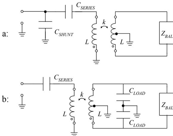
**Figure 3: Two balun/matching network circuits.**
