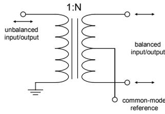
**Figure 1: Transformer-based balun**
