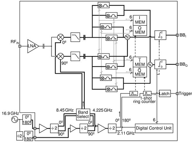
Fig. 2. Block diagram of the double-conversion receiver with digital IF correlators (thick lines indicate differential signal paths).
