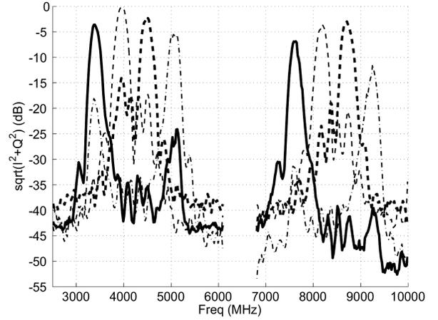
Fig. 5. Pulse receiver response to swept sinusoidal RF input when correlating with the corresponding template with time-limited sinc-shaped envelope for the 8 different channels.
