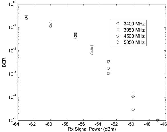
Fig. 8. Measured BER versus receiver signal power at 50 Mb/s using OOK modulation for different channels.
