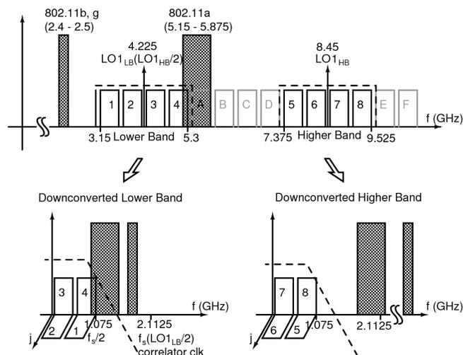
Fig. 1. Frequency plan of the pulse radio receiver before and after the first wideband downconversion, shown with existing 802.11 WLAN interferers.
