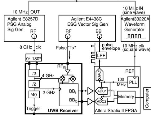
Fig. 6. UWB receiver BER measurement setup for 50 Mb/s OOK demodulation.
