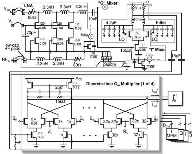
Fig. 3. Schematics of the LNA, mixer, filter and  $G_m$ -multiplier.
