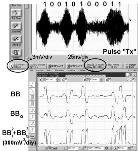
Fig. 7. Input UWB pulses and quadrature receiver outputs demodulating an OOK signal at 50 Mb/s; each input pulse is correlated twice and therefore produces two identical outputs for each bit (see text).
