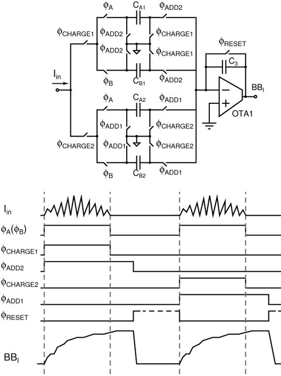
Fig. 4. Single-ended equivalent schematic of the rotating switched-capacitor windowed integrator and its timing diagram.
