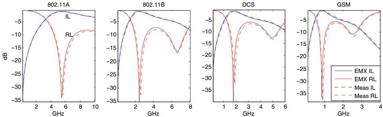
Figure 7: Insertion loss (IL) and return loss (RL) of baluns: EMX simulation vs measurement
