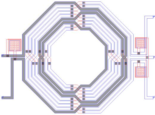
Figure 2: 1:2 Balun layout with MIM capacitors
