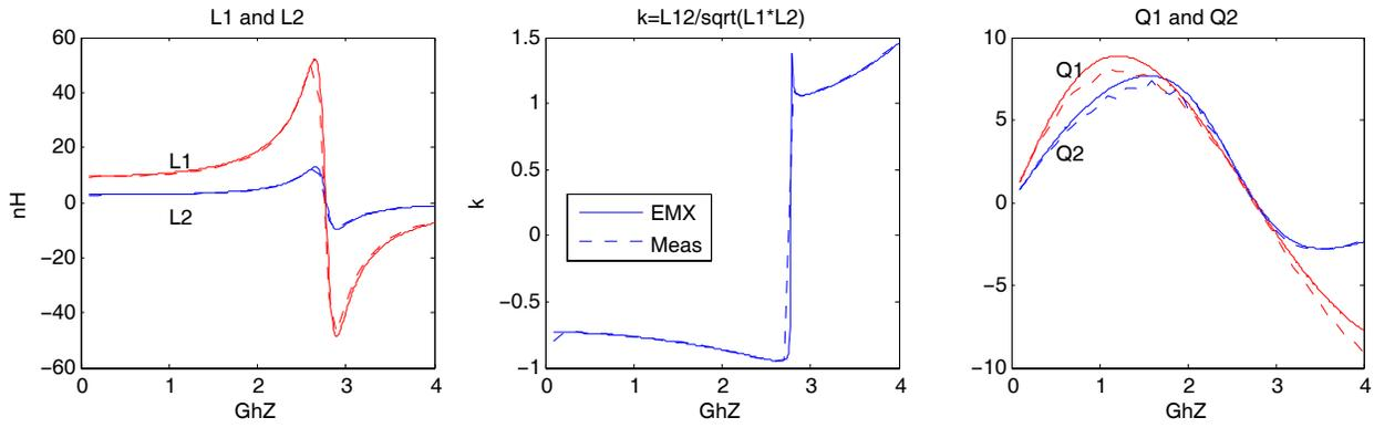
Figure 6: Inductance,  $k$ , and  $Q$  of the DCS transformer: EMX simulation vs measurement
