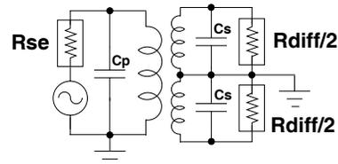
Figure 1: Balun schematic
