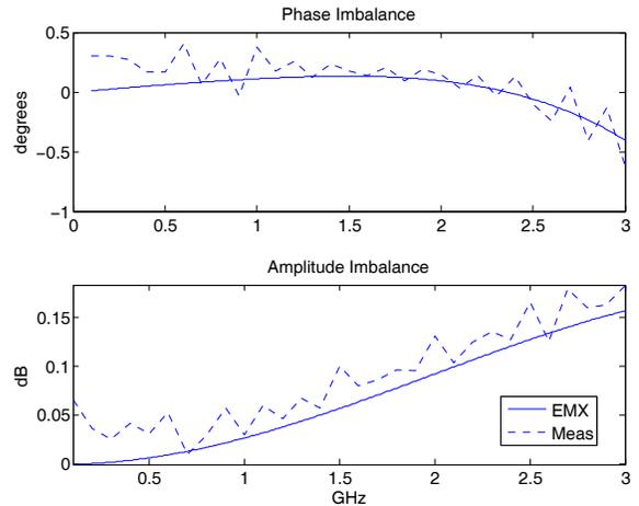
Figure 8: Amplitude and phase imbalance of DCS Balun: EMX simulation vs measurement
