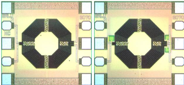
Figure 5: Transformer and balun in padframe
